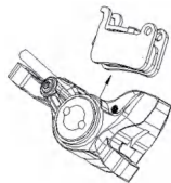
Figure 2-5 Removing/Assembling the Brake Pads and Accessories
