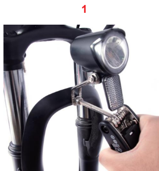
1. Pre-install the headlight and the fender on the front fork with the headlight fixing screws.
