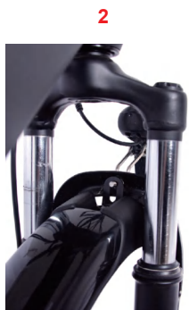
2. Tighten the screw with the No. 5 Allen key in the 16-in-1 tool.
